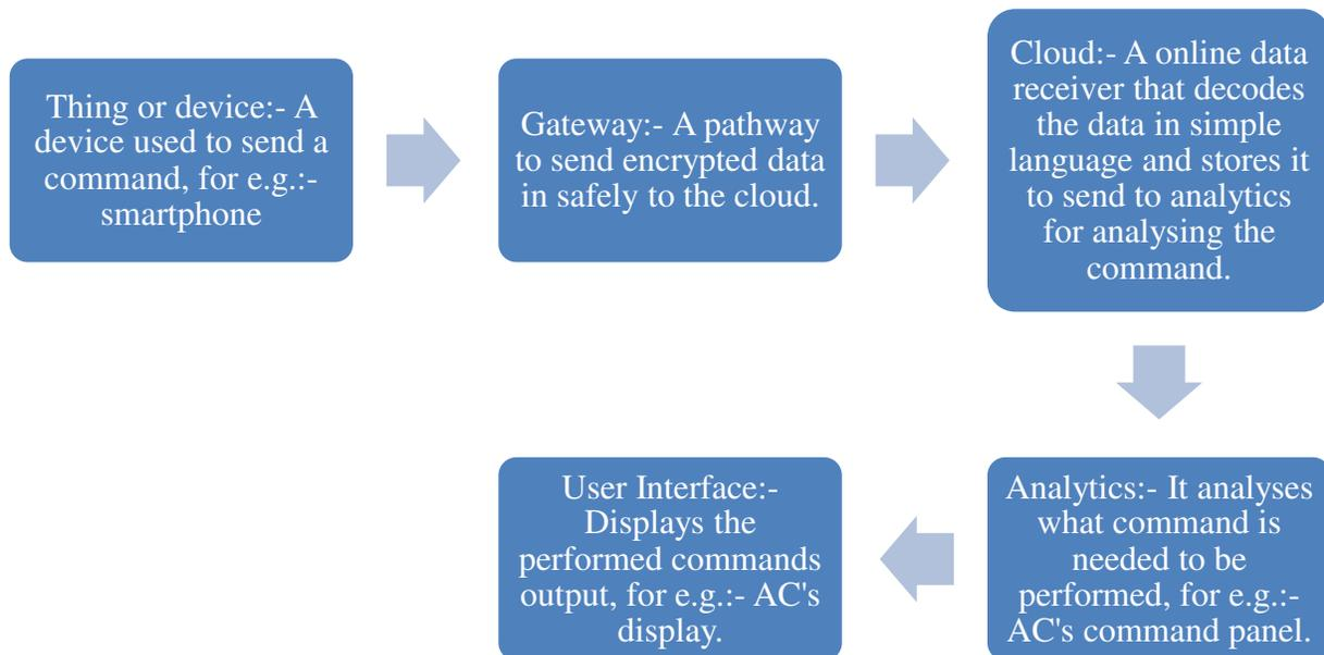
But it does require various things like sensors and to detect the need of the user and the environmental conditions to send a valid command data. It needs actuators to understand the entered command and start the processing of data in the hardware mechanism. Connectivity, which can be through Wi-Fi, Bluetooth, Mobile data, or any other specific authorized network.
